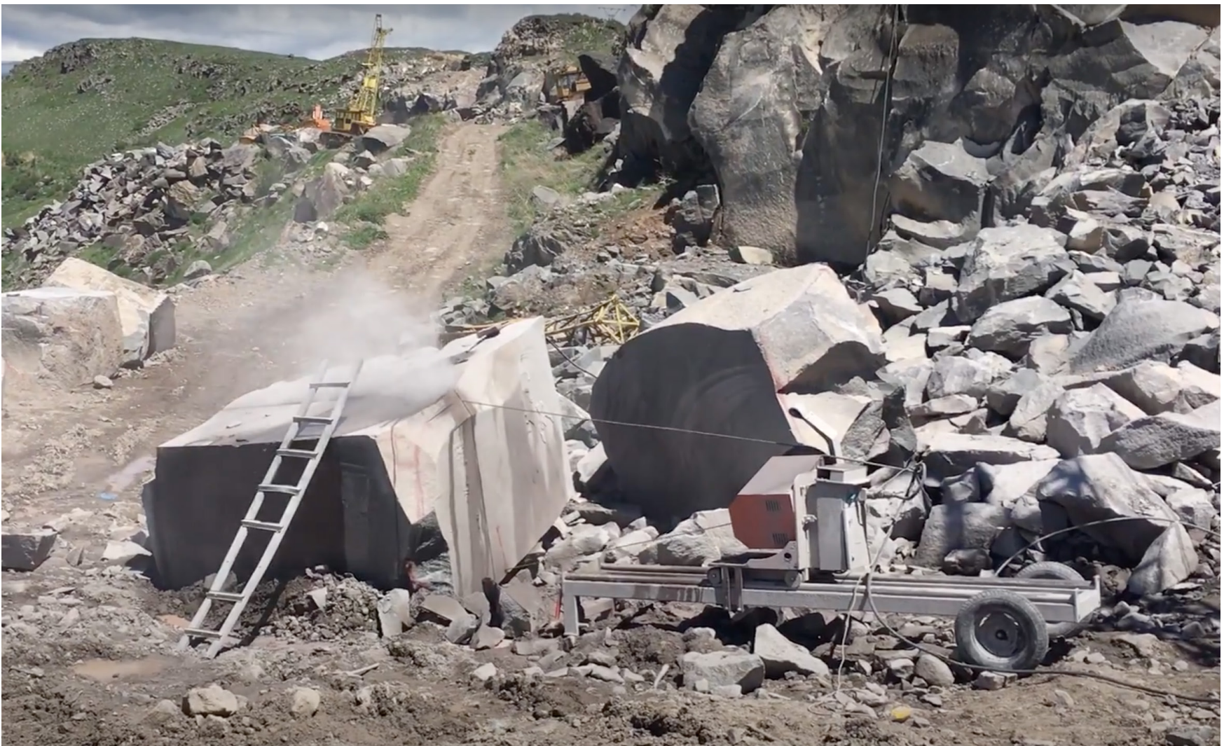
Squaring blocks with a diamond wire saw
