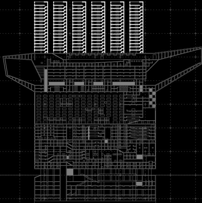
Concrete cores are placed with the highest possible construction height that can be achieved within the system. They are reminiscent of the towers of Kollhoff's design, but follow a static principle.
