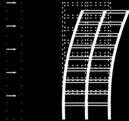
A Belltruss and Outrigger System reduces the yield factor to a minimum for wind loads.
