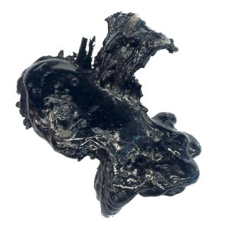
A viscous, black petroleum byproduct that acts as a binder, holding together aggregates and giving asphalt its characteristic waterproofing properties. Bitumen is essential for the flexibility and adhesive properties of asphalt.
